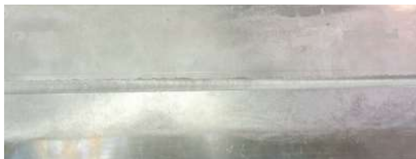
Fig.2 Welded joint of Al –alloys (5052 H34 with7075 T6)
