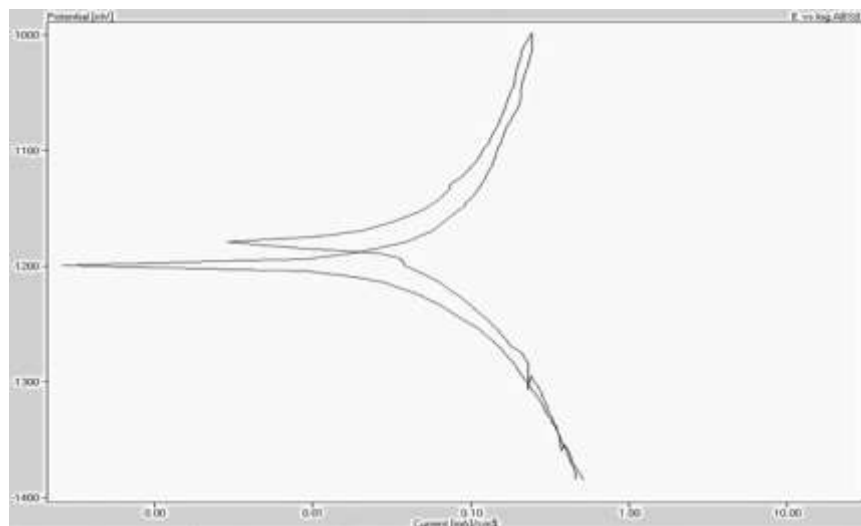
Fig.13 Cyclic polarization for base alloy 5052-H34 in 0.5% NaOH
