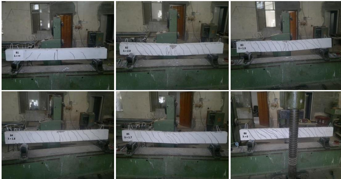
Figure 9: Failure of the tested beams
