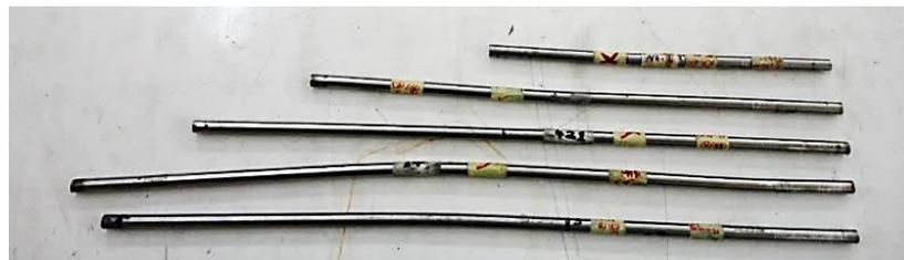
Figure 4. Specimens before and after buckling test.
