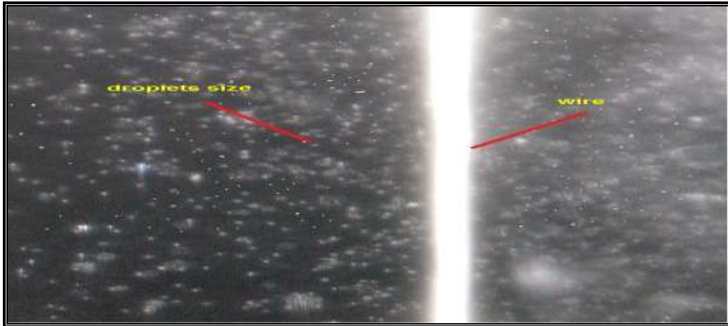
Figure (5): Photography showing the fuel droplets size for comparison with the wire diameter.
