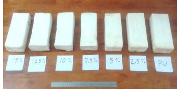
Figure 1. Cast of Polyurethane foam with polypropylene fibers composite.
