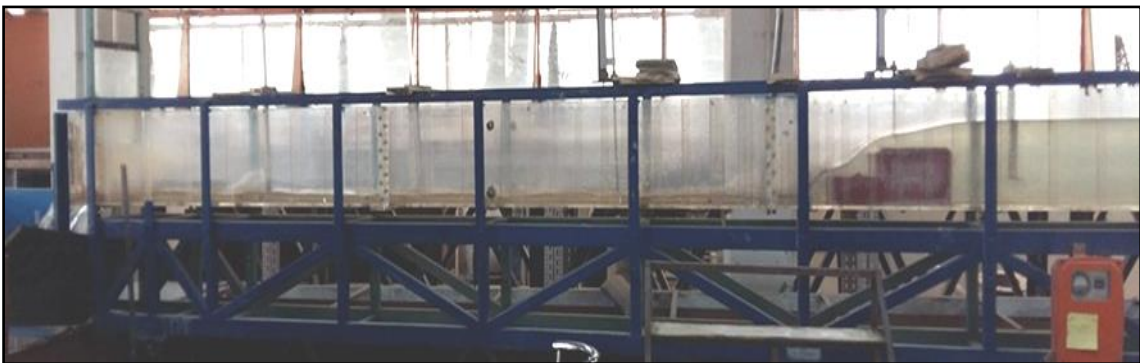
Photo A. The Laboratory Flume with Broad Crested Weir
