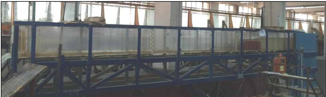
Photo A. The Laboratory Flume with Broad Crested Weir
