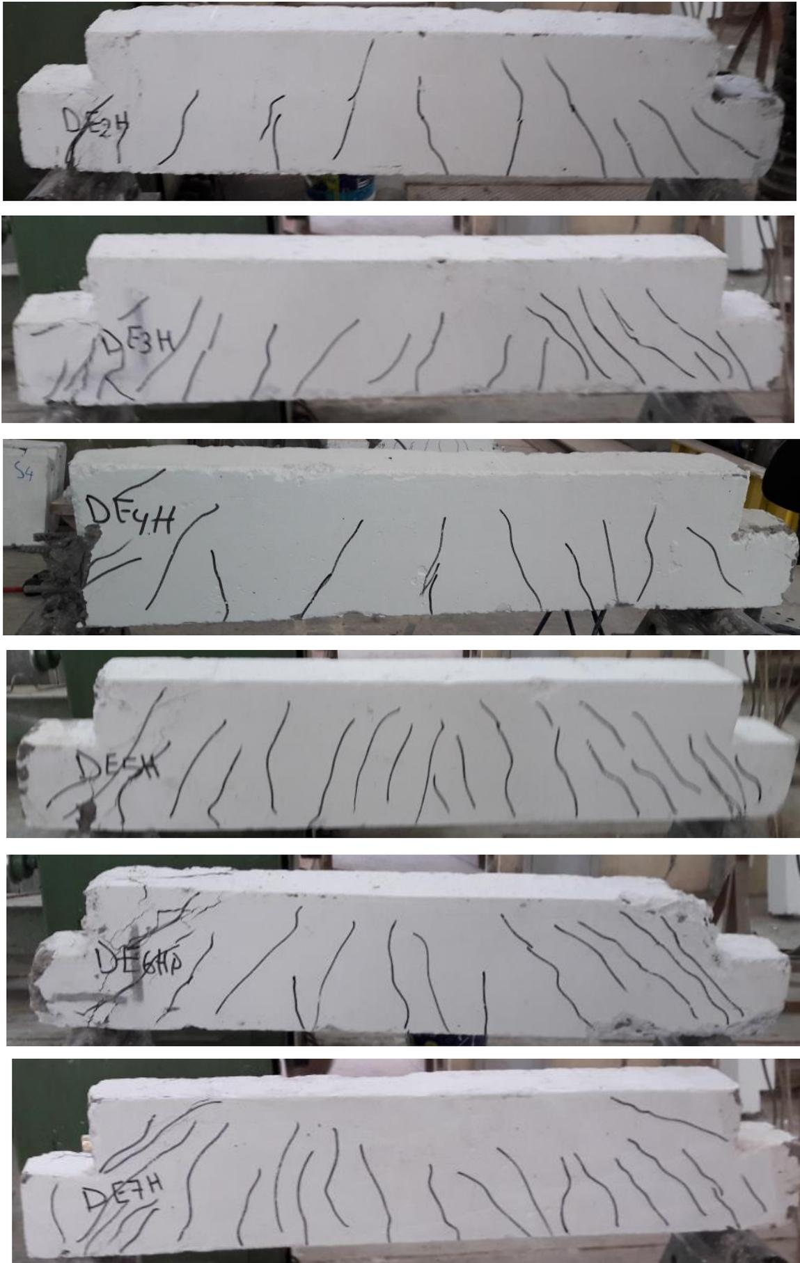
Fig. (8). Crack Pattern of All R.C. Inverted Dapped Ends Beams.
