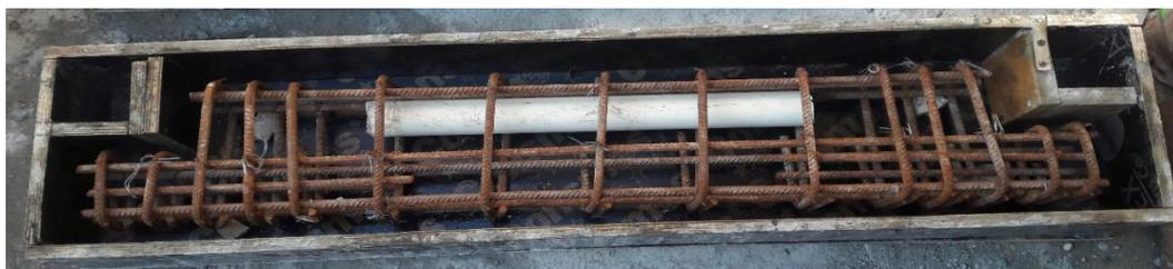
2. Mould & Reinforcement of R.C. Inverted Dapped Ends Girder, (DE2H)
