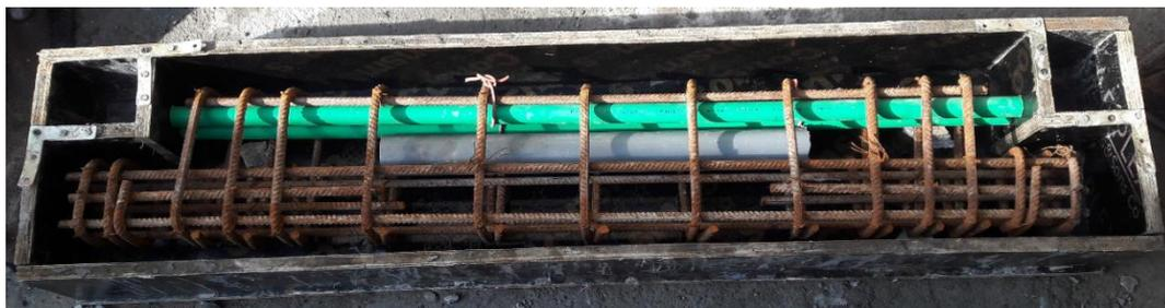
6. Mould & Reinforcement of R.C. Inverted Dapped Ends Girder, (DE6HP), Double Bolts.
