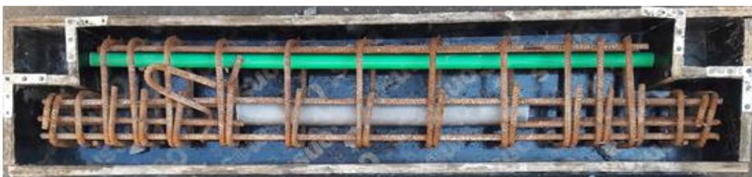
7. Mould & Reinforcement of R.C. Inverted Dapped Ends Girder, (DE7HP), Double Bolts.
