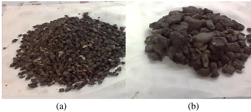
Plate 1. Samples of the Recycled Asphalt Pavement. a) Fine RAP b) Course RAP
