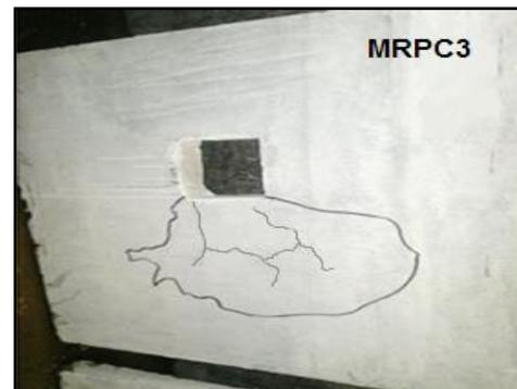
Plate 10. Tension Face for Slab MRPC3
