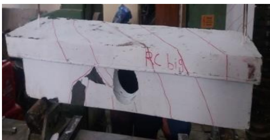
Plate 12. Specimen beam B9 – after test.
