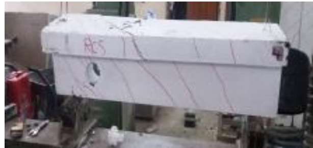
Plate 7. Specimen beam B4 – after test.
