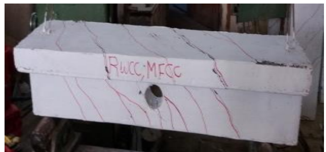
Plate 13. Specimen beam B10 – after test.
