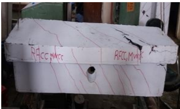
Plate 10. Specimen beam B7 – after test.
