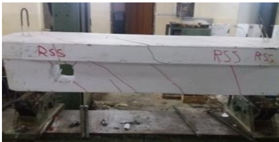
Plate 8. Specimen beam B5 – after test.
