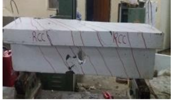
Plate 5. Specimen beam B2 – after test.
