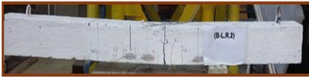
Fig.8, Cracks Pattern of the RPC Beam (B-L.R.2)
