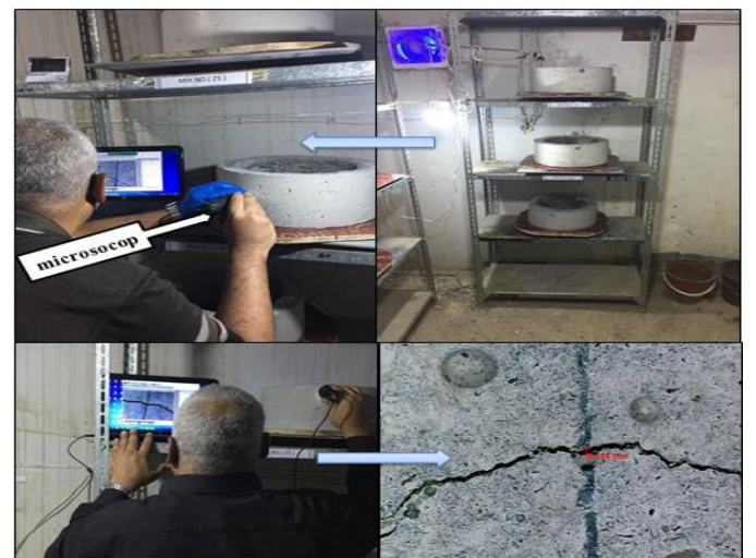
Plate 3. Reading Crack width for Ring
