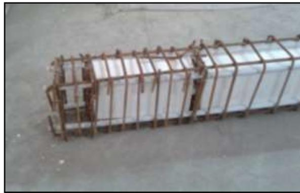
Plate 1. Reinforcement Details and Diaphragms Location
