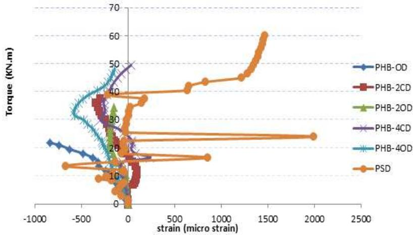
Figure 11. Concrete Strains (Location-2)
