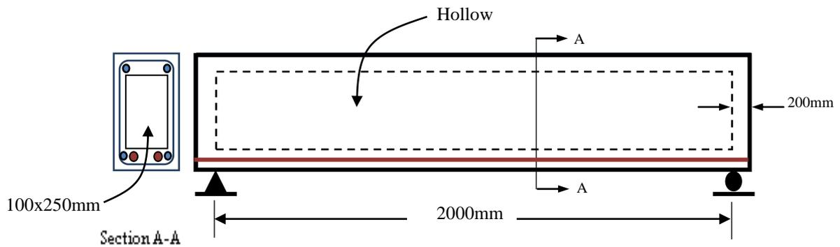
Figure 2. Description of Beam Specimen (PHB-0D)
