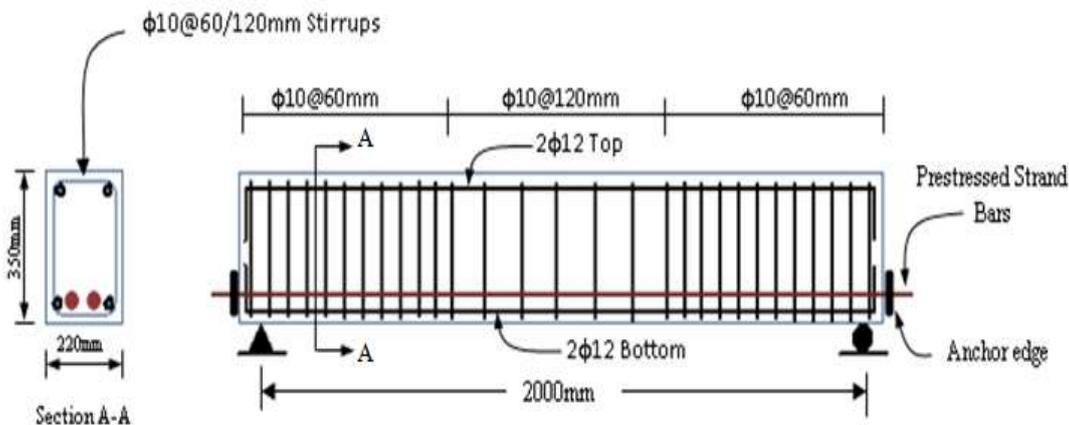
Figure 1. Reinforcement Details and Dimensions of the Tested Beams
