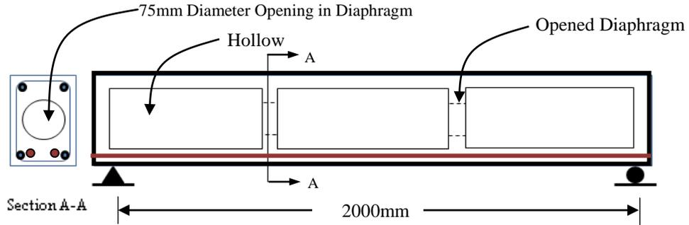
Figure 4. Description of Beam Specimen (PHB-2OD)
