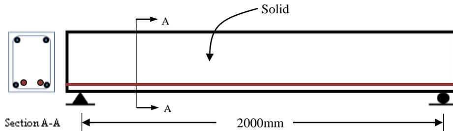
Figure 7. Description of Beam Specimen (PSB)
