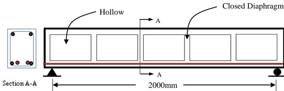
Figure 5. Description of Beam Specimen (PHB-4CD)
