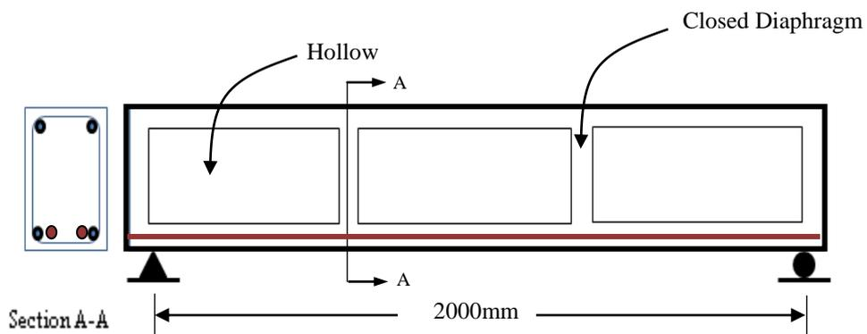
Figure 3. Description of Beam Specimen (PHB-2CD)
