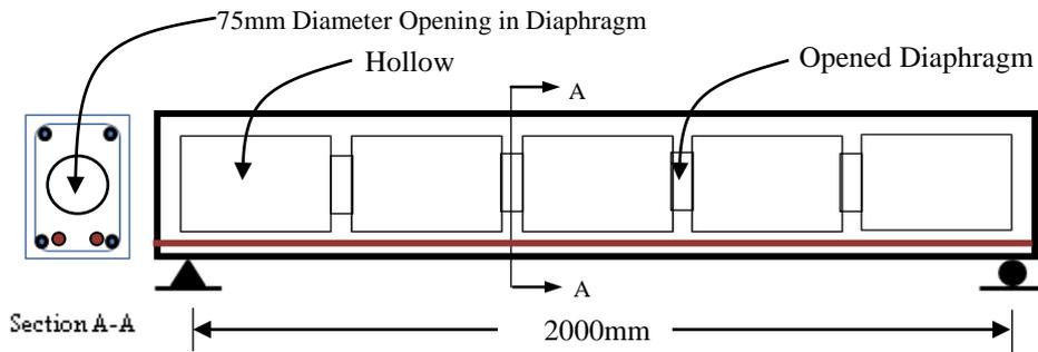
Figure 6. Description of Beam Specimen (PHB-4OD)
