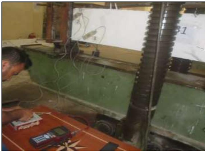
Plate 6. Strain Gauges and Data Logger Setup
