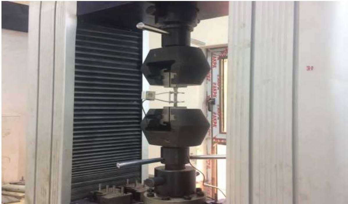
Figure 1. The universal testing machine used to make tensile test.
