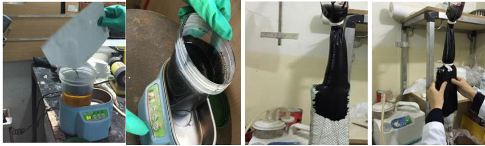
Figure (8): Adding the mixture of CNTs, resin and hardener from the hole above molding.
