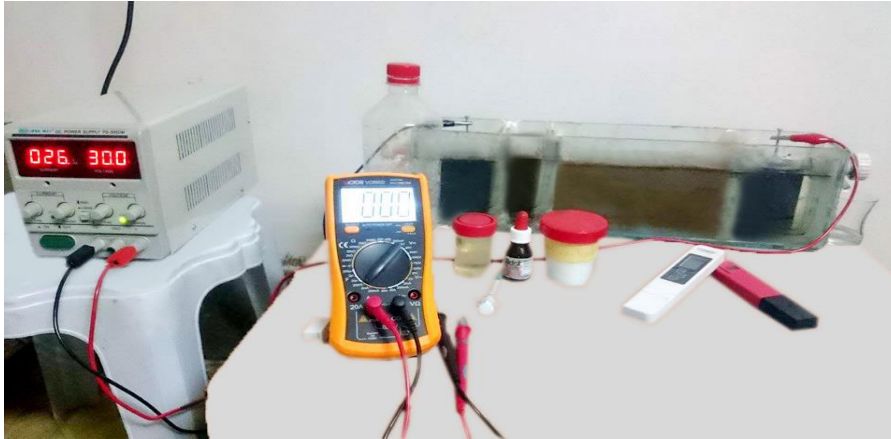
Figure.2 Experimental set-up of electro-kinetic cell.
