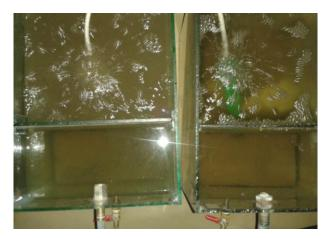
Figure 4. Top view showing the settlement of the biomass in the aeration tank
