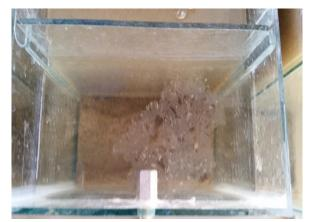
Figure 5. Top view of the final clarifier showing filamentous bacteria
