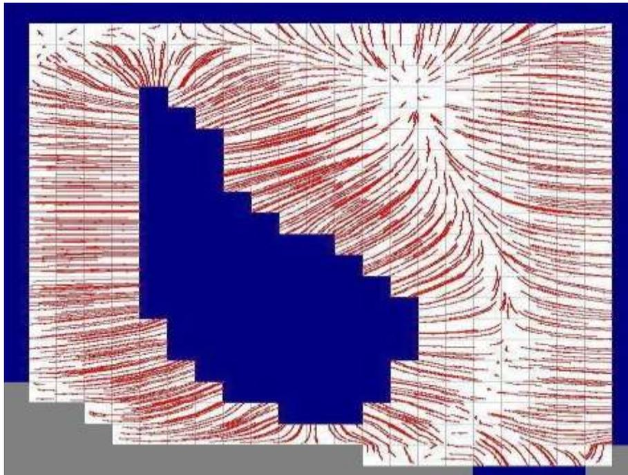
Fig.(15)Flow Paths of Ground Water That Discharge to Tharthar Lake.
