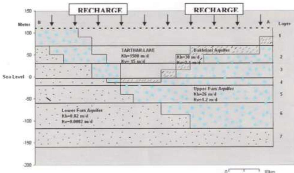
Fig.(9): vertical discretization, boundary condition, and calibrated hydraulic conductivity for simulation model of the groundwater flow system near tharthar lake, cross-section AB location is shown in Fig.(3).
