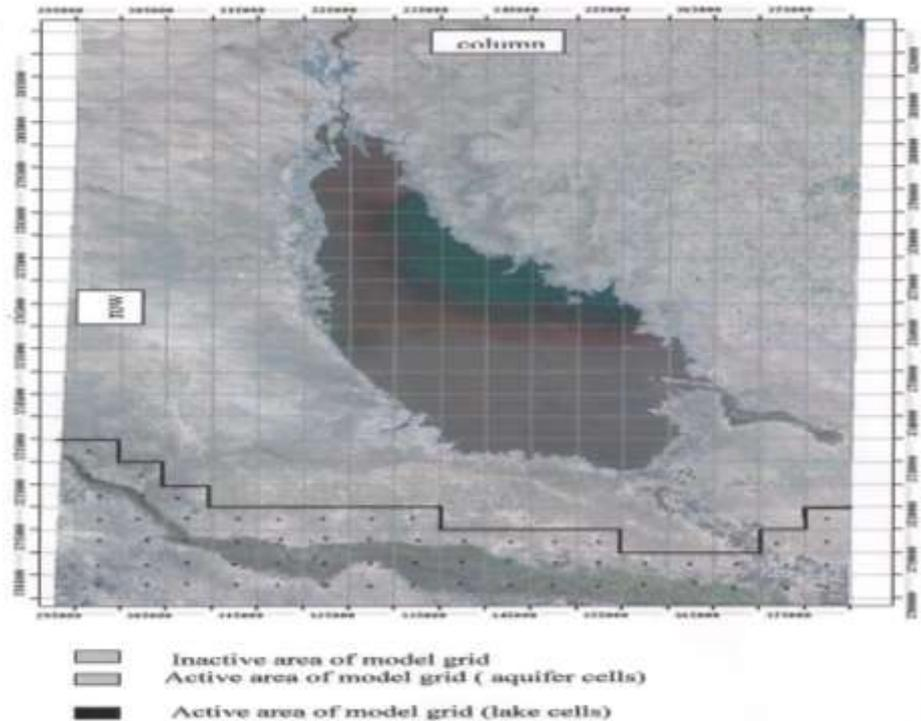
Fig.(8): area discretization and boundary condition for simulation models of groundwater flow near tharthar lake.
