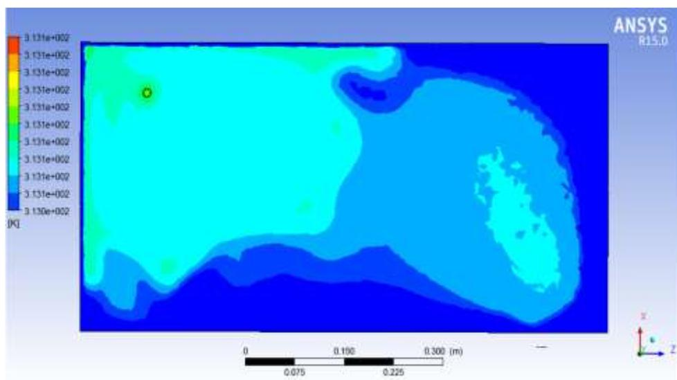
Figure 5. temperature distribution x-z plane top view at x=330 mm from the bottom case1
