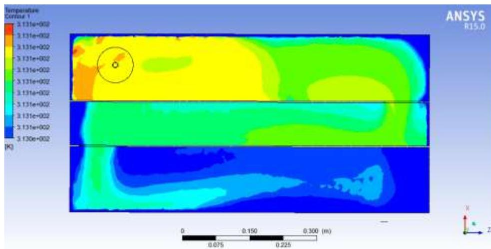
Figure 9. Temperature distribution x-z plane top view at x=330 mm from the bottom case 3
