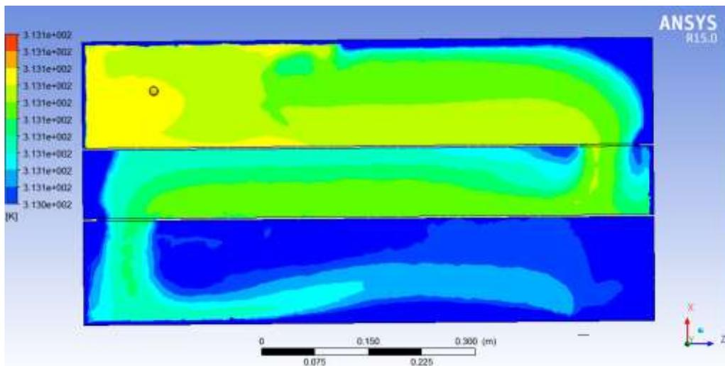
Figure 7. temperature distribution x-z plane top view at x=330 mm from the bottom case 2
