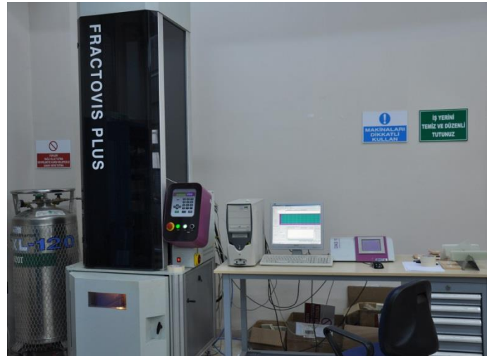
Figure 3 Fractovis Plus impact machine with data acquisition system (DAS)
