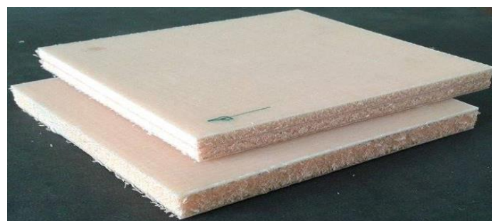
Figure 2. Prepared specimens of sandwich composites (a) with multi core (b) normal
