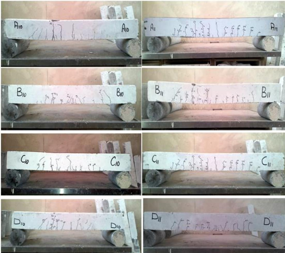
Fig. (9) Crack pattern for tested beams.
