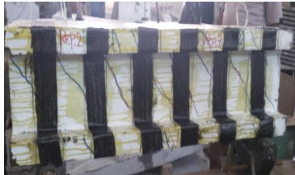
Figure (16): repaired of composite beam (Rep2)
