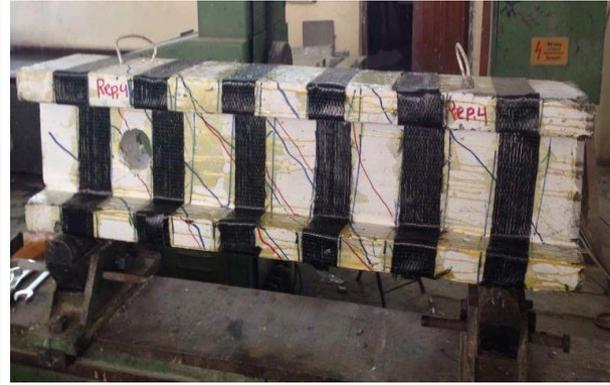
Figure (20): repaired composite beam (Rep4)
