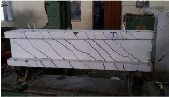
Figure (13): unrepaired composite beam (B1)
