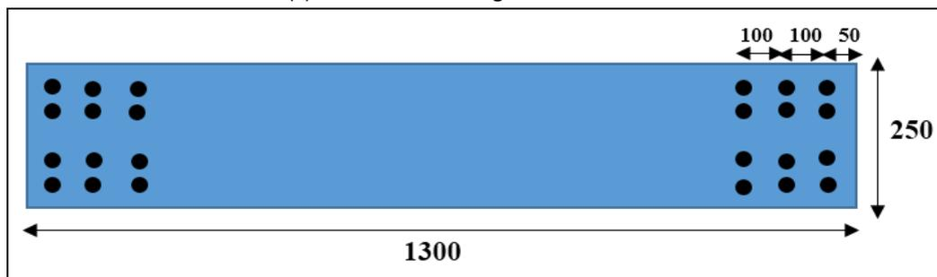
Figure (2) Details of steel plate with shear connector (Bottom view) (all the dimension in (mm))
