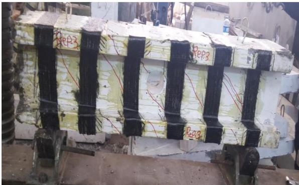
Figure (18): repaired composite beam (Rep3)
