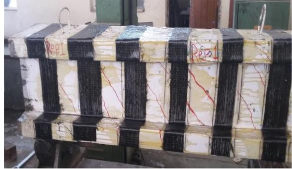
Figure (14): repaired of composite beam (Rep1)
