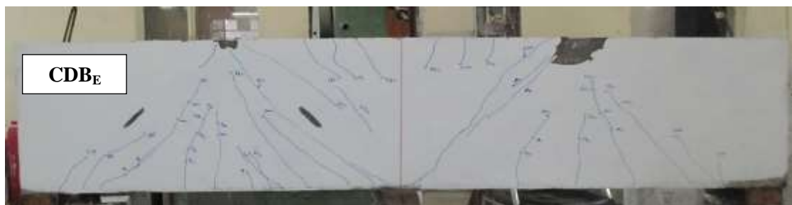
Figure 12. Crack pattern for beam CDB e after testing.
