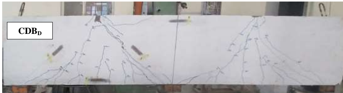
Figure 11. Crack pattern for beam CDB d after testing.
