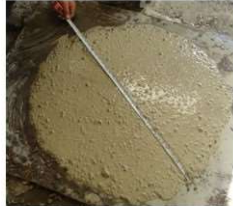
Figure 6. Spreading concrete in Slump Flow test of SCC.
