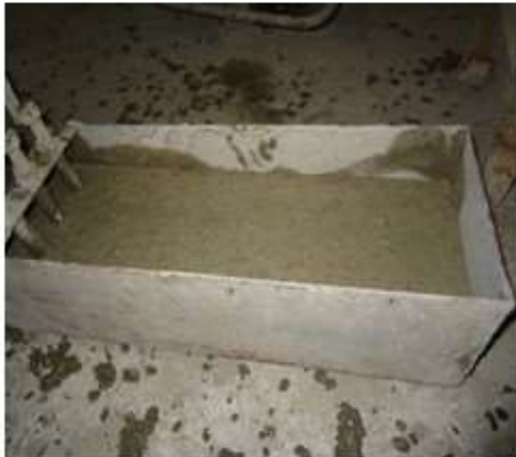
Figure 5. Flowing of concrete in horizontal section in L-box test of SCC.
