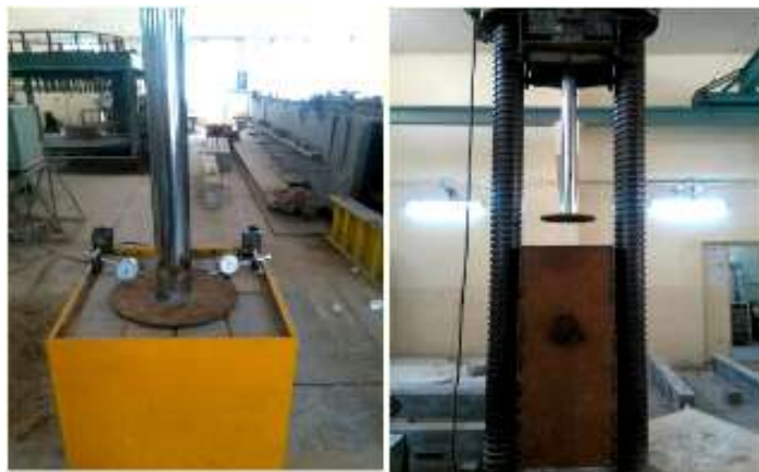
Figure (4) Static plate load test setup
