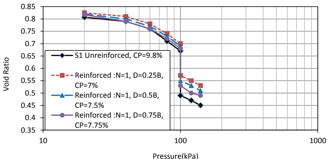
Figures (11). The relationship between the pressure and void ratio for soil (S1)
