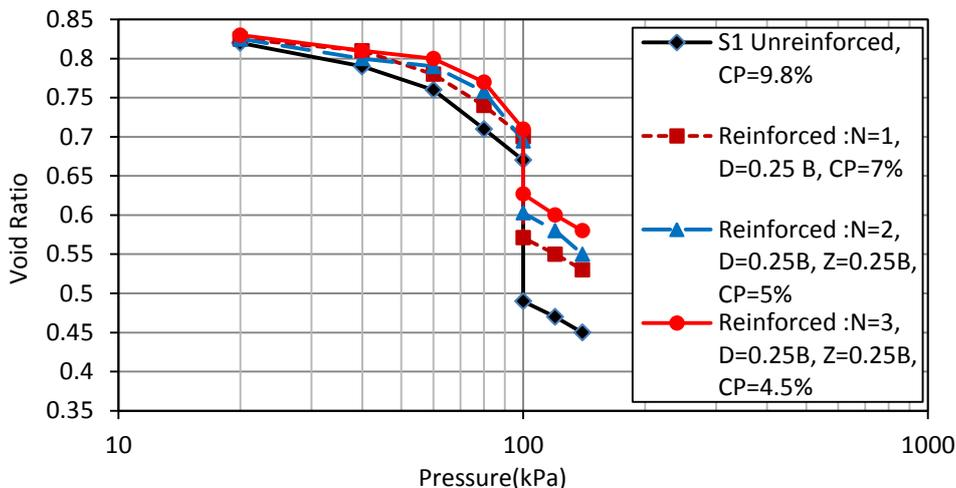
Figures (14). The relationship between the pressure and void ratio for soil (S1)
