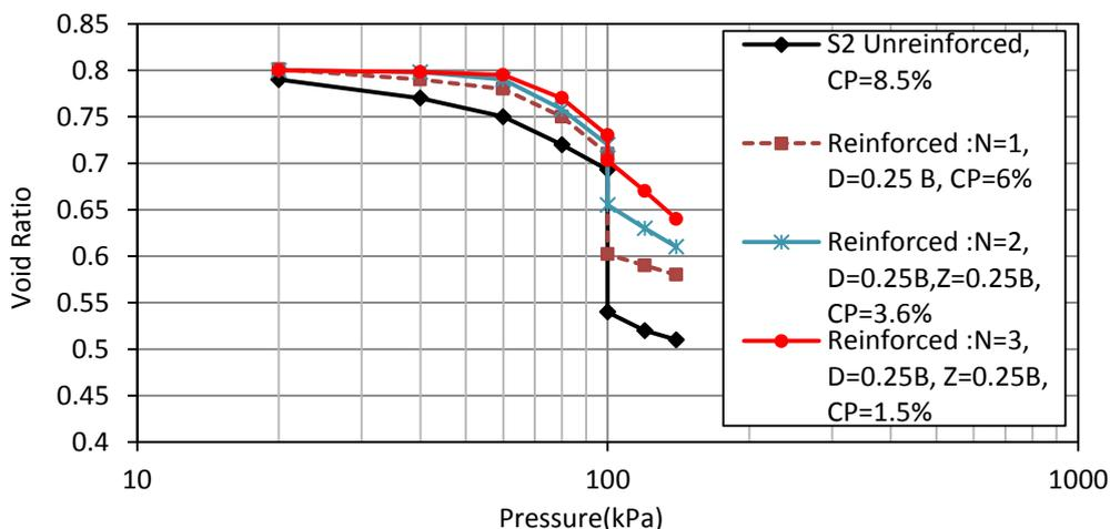
Figures (15). The relationship between the pressure and void ratio soil (S2)
