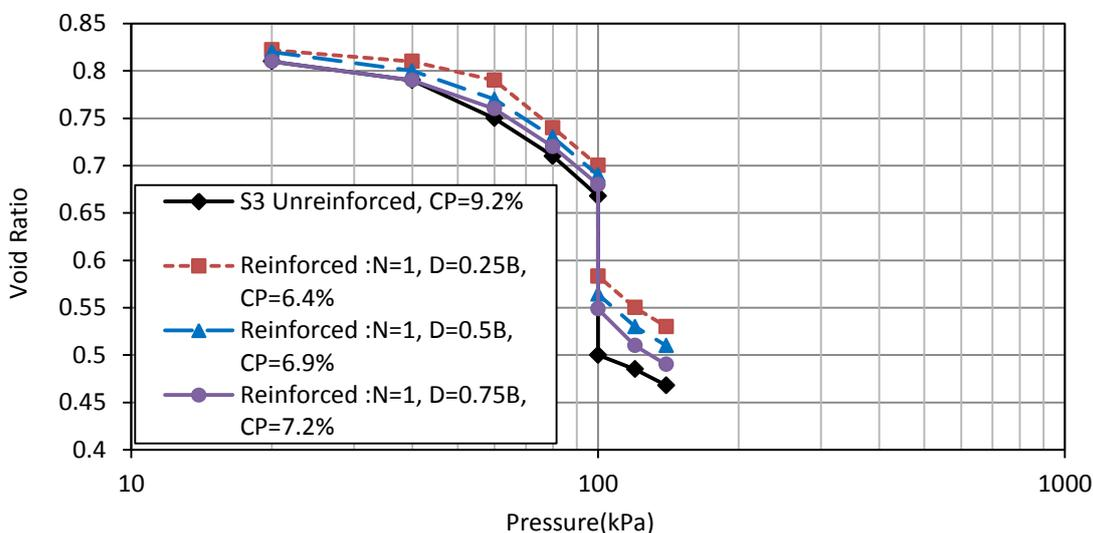
Figures (13). The relationship between the pressure and void ratio for soil (S3)
