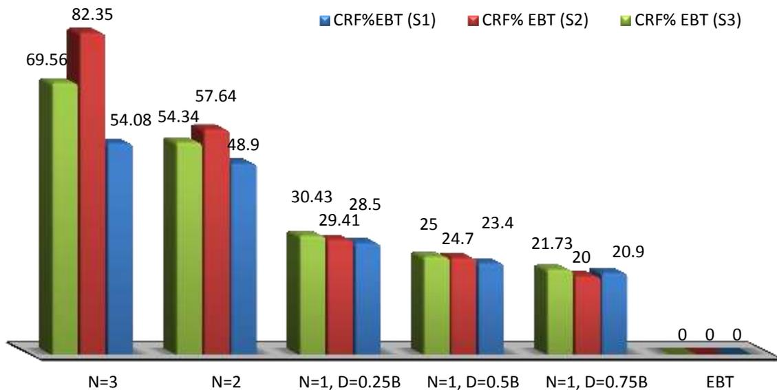
Figure (20). The improvement as (CRF) in gypeuos soils with respect to (EBT)
