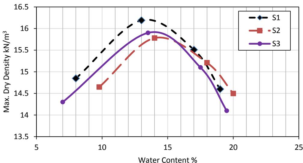
Figure (4). Compaction Curves for Soils S1, S2 and S3
