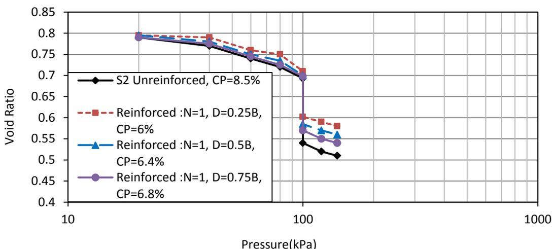
Figures (12). The relationship between the pressure and void ratio for soil (S2)
