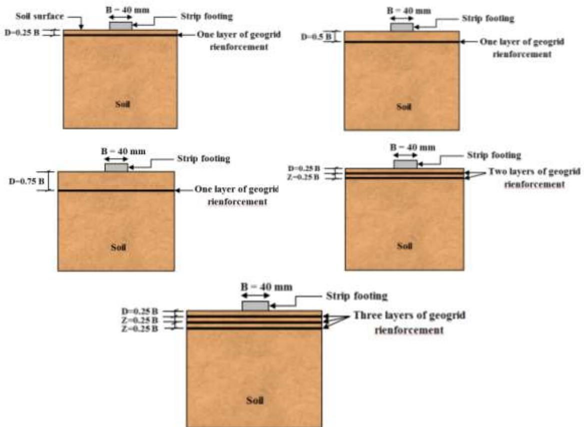
Figure (10). The position and the number of the reinforcement layers
