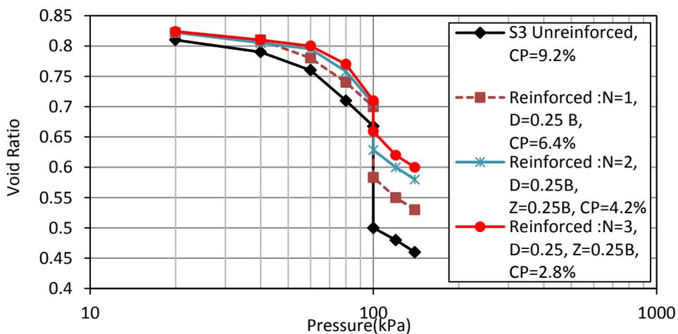
Figures (16). The relationship between the pressure and void ratio for soil (S3)
