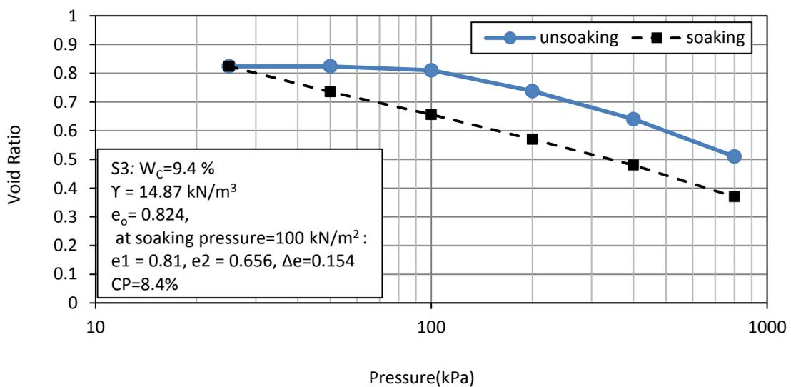
Figure (7). Typical results of collapse test (CT) for soil S3
