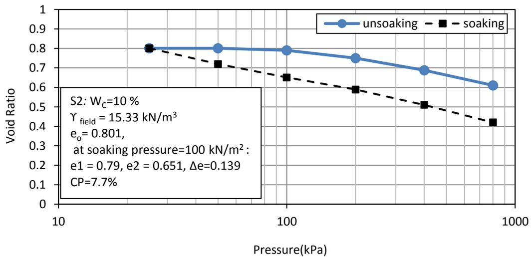
Figure (6). Typical results of collapse test (CT) for soil S2
