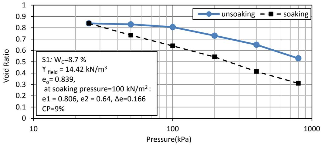
Figure (5). Typical results of collapse test (CT) for soil S1
