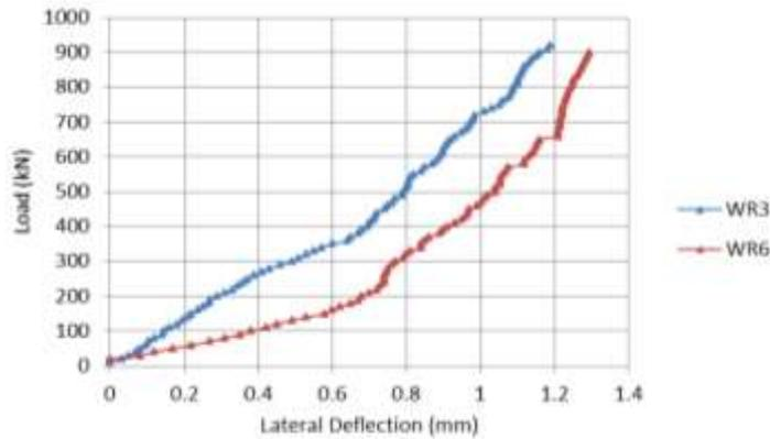
Fig (7) : Effect of ( $\rho$ ) on Load-deflection Behavior With (AR=2.00).
