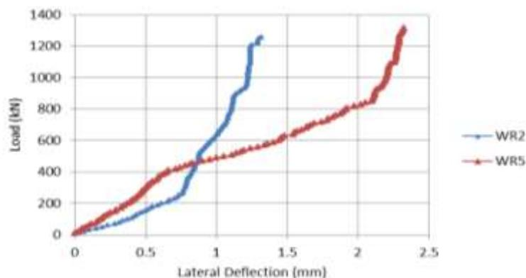
Fig (6): Effect of ( $\rho$ ) on Load-deflection Behavior with (AR= 1.50).
