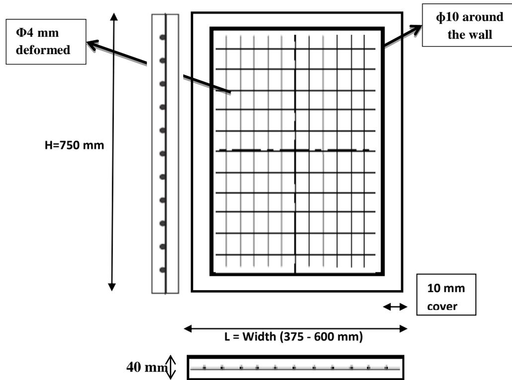
Figure (1): Arrangement of Reinforcement in Panel.
