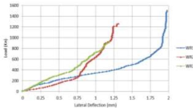
Figure (3): Effect of AR on Load-deflection Behavior for RPC With  $\rho = 0.012566$ .
