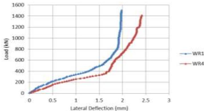
Fig (5): Effect of ( $\rho$ ) on Load-deflection Behavior with (AR= 1.25).
