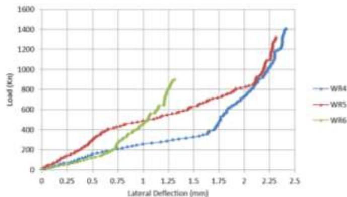
Figure (4): Effect of AR on Load-Deflection Behavior for RPC with  $\rho = 0.007854$ .
