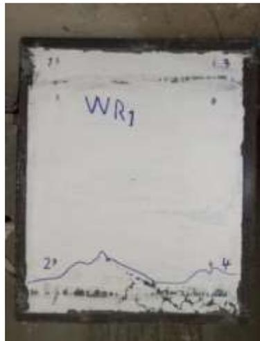
Plate (3)B:WR1 Tension Face.
