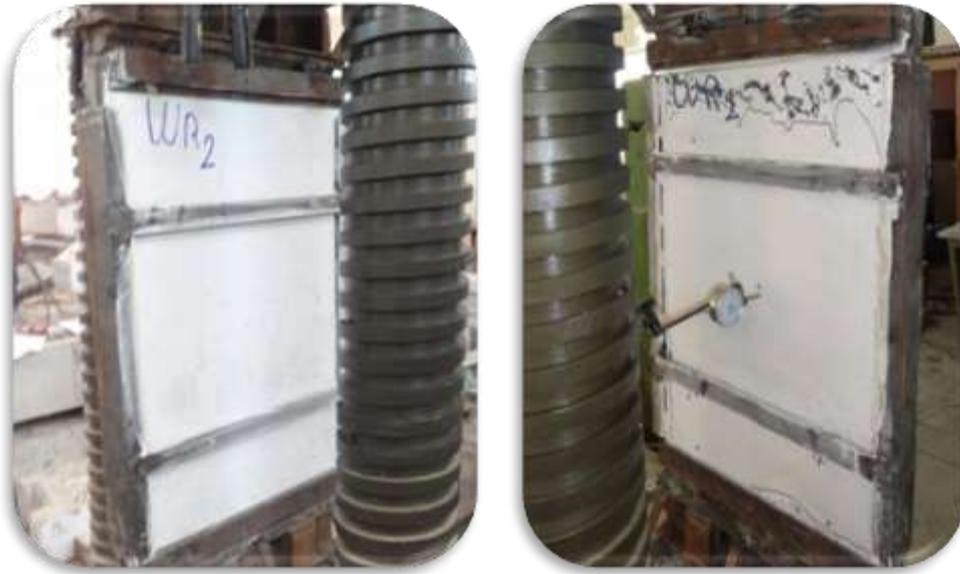
Plate (2): RPC Wall Panels Before and After the Test.
