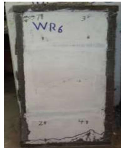
Plate(8)B:WR6 Tension Face.
