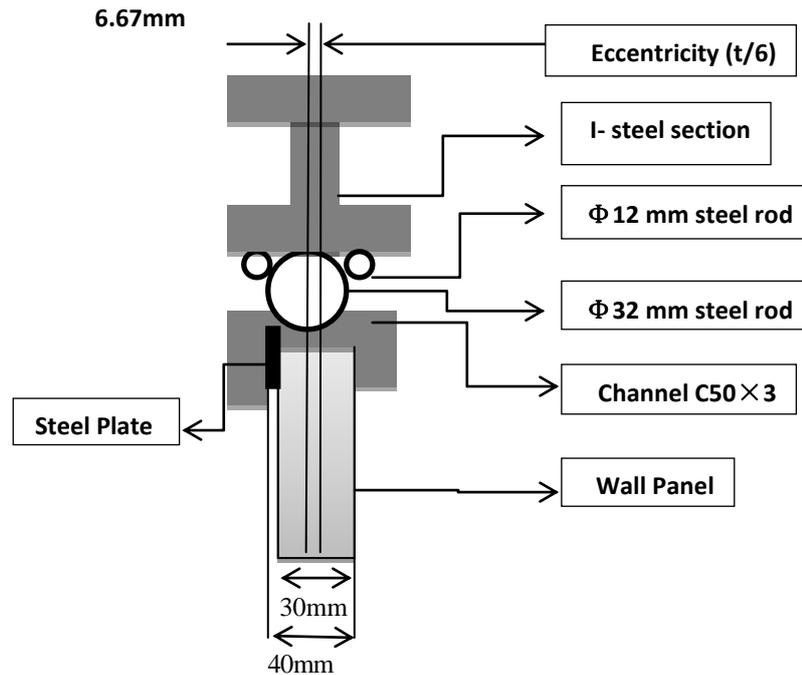
Figure (2): Detail of Supports Used In this Work.
