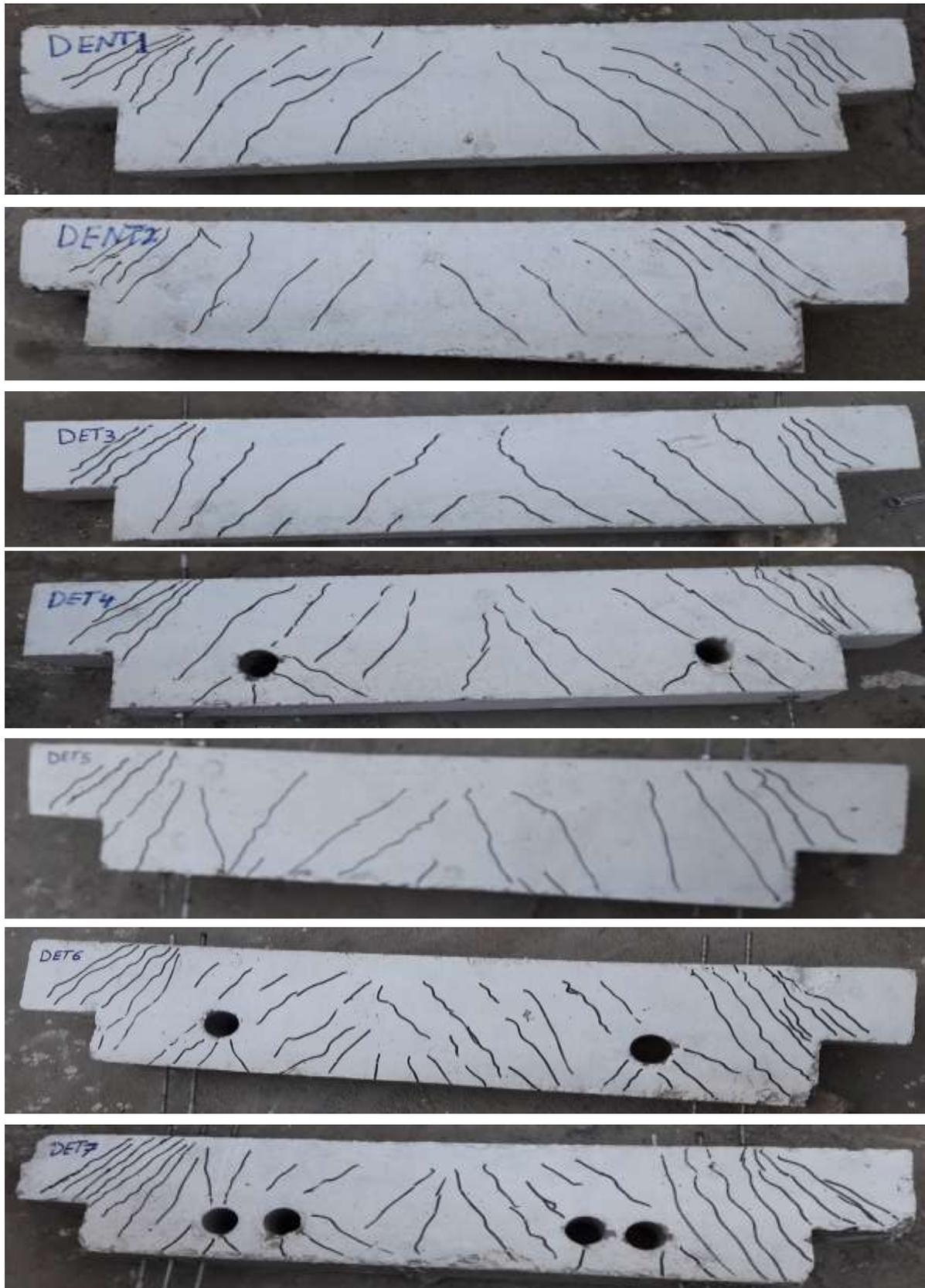
Fig. (8). Crack Pattern of Tested Beams.
