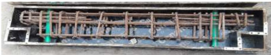
(C) Mold and Reinforcement of R.C. Beam Dapped Ends, (DE3).
