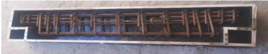
(B) Molds and Reinforcement of R.C. Beam Dapped Ends, (DE1 & DE2)
