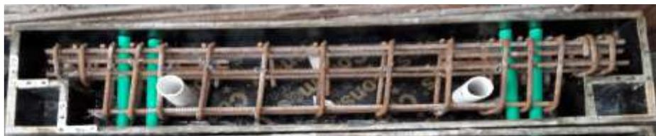
(F) Mold and Reinforcement of R.C. Beam Dapped Ends, (DE6).
