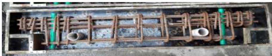
(D) Mold and Reinforcement of R.C. Beam Dapped Ends, (DE4).
