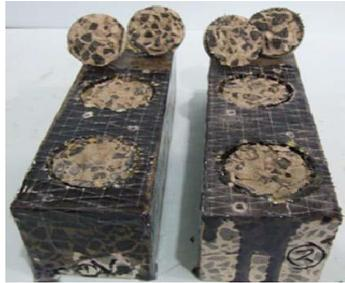
**Figure 5.** Failure mode of CFRP/concrete system at ambient conditions [33]
