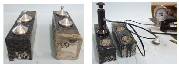
**Figure 1.** Adhesion pull-off test at ambient conditions for ES FRP/concrete system using EBA [33]
