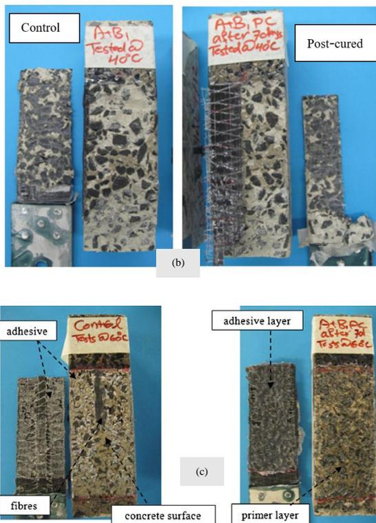
**Figure 16.** Failure modes for ES CFRP/concrete system using EBA with and without post-curing at 60°C and tested at: (a) moderate elevated temperatures and constant load, (b) 40°C and (c) 60°C [49]
