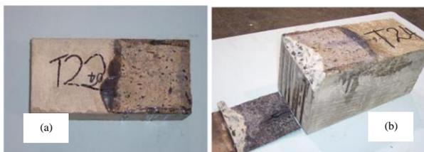
**Figure 15.** Failure modes for ES CFRP/concrete system using EBA at elevated temperatures [48]
