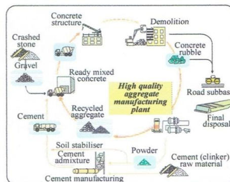
Figure 1: Schematic flow of concrete recycling system ( Hirokazu, et.al, 2005)
