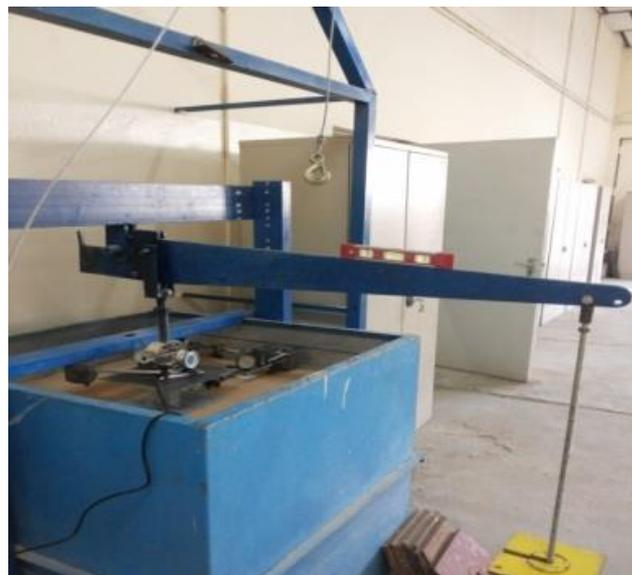
Figure 2: Loading frame and sand box.
