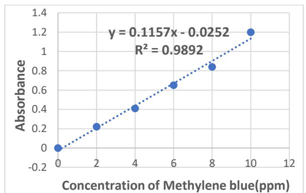
Figure 5. Calibration curve for MB in ppm
