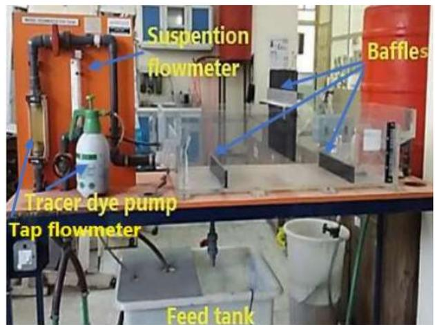
Figure 1. Laboratory sedimentation tank model
