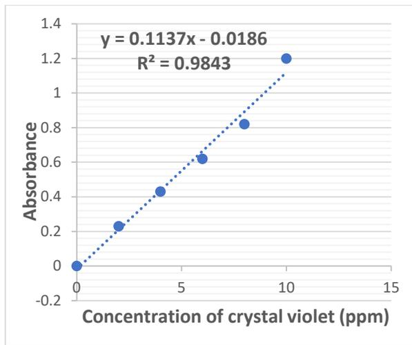
Figure 6. Calibration curve for CV in ppm
