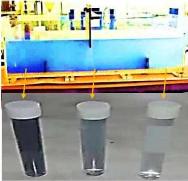
**Figure10.** Dye graduated through the sedimentation tank areas
