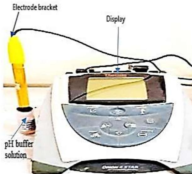
Figure 3. Thermo Orion 4-star pH ISE Benchtop meter
