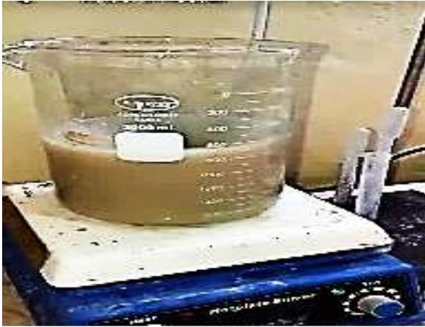
**Figure 7.** Mixing kaolin using a Hotplate Stirrer
