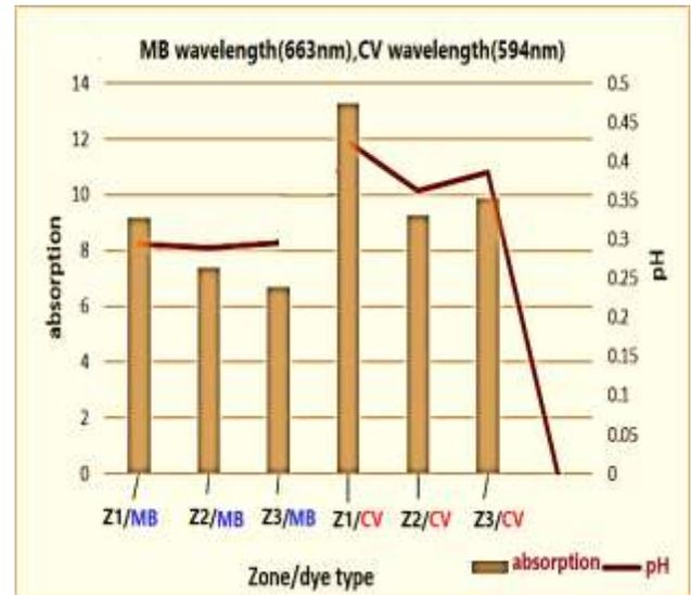
**Figure 8.** Relationship between pH and absorption and its change with two cationic(basic) dyes inside three zones of the sedimentation tank at temperature 25 °C
