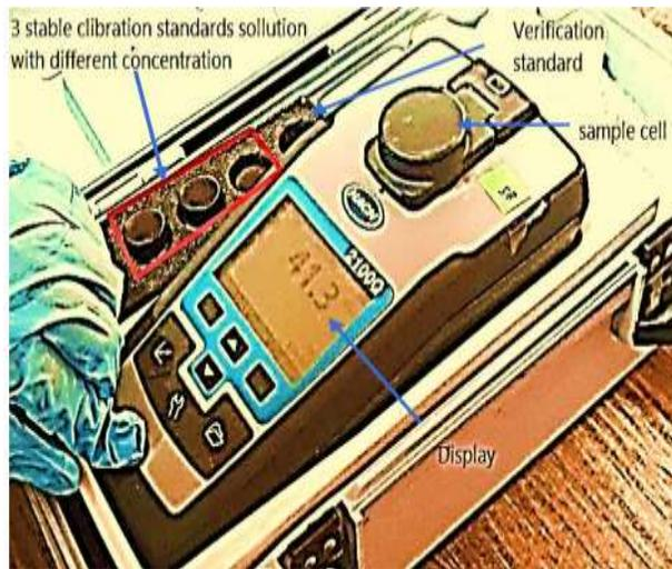
Figure2. Hatch 2100Q turbidity meter
