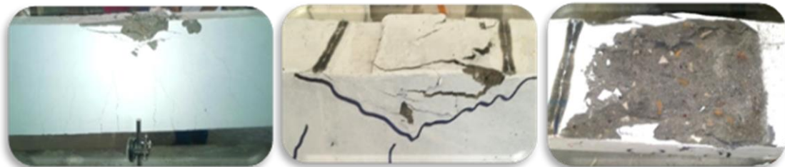
Fig. (13): Concrete Crushing Failure in Upper Layer of Some Beams
