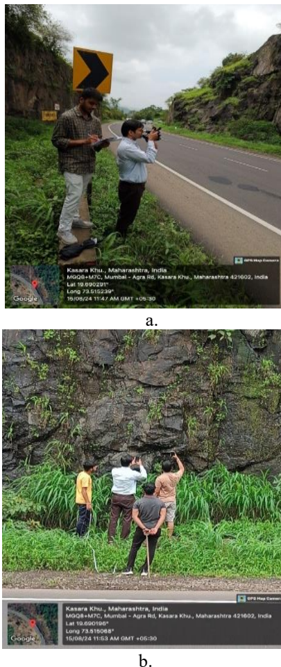
Figure 3. Field measurements using a nautical sextant.
