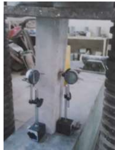
Figure 5. Column specimen setup.
