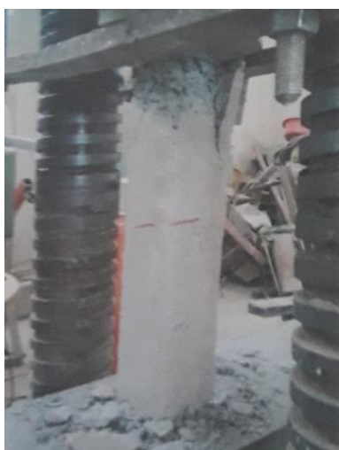
Figure 11. Crack pattern of specimen C3 after testing and failure Mechanism.
