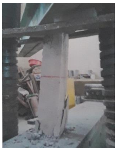
Figure 12. Crack pattern of specimen C4 after testing and failure Mechanism.
