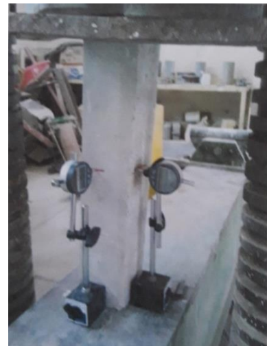
Figure 5. Column specimen setup.
