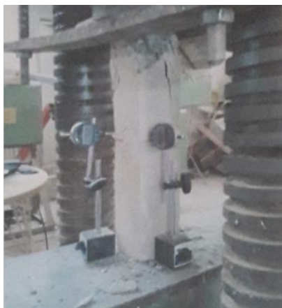
Figure 10. Crack pattern of specimen C2 after testing and failure Mechanism.
