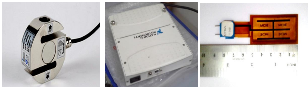
Figure 5. a) Load cell S-type SS-300, b) NI DAQ Pad-6015 data Acquisition device, c) Piezo- actuator and sensor type QP16N, film thickness 0.01 in.
