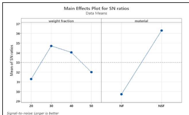
Figure 12. The analysis of tensile and bending strength results by the Taguchi method for natural NF and hybrid NSF fibre composites.
