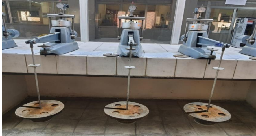
Figure 1. Collapse test for gypseous soil samples under test.
