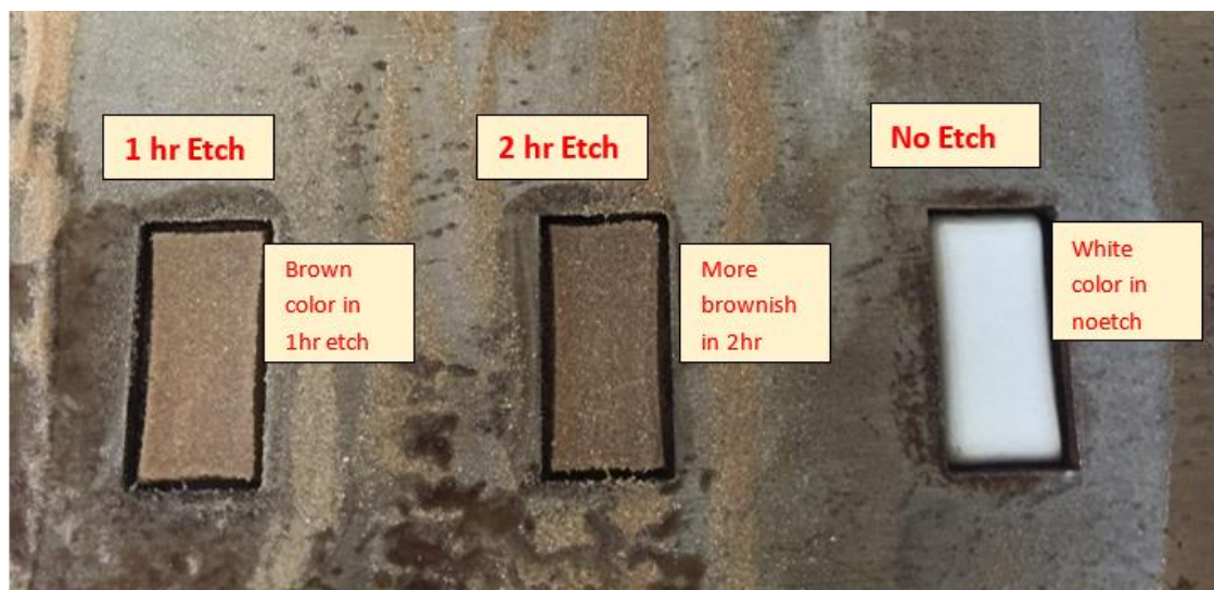
Figure 2. Polyamide 12 surface color changes: natural (no etching), brown (1-hour etching), and darker brown (2-hour etching).
