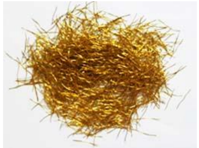
Figure 1. Used steel fibers.
