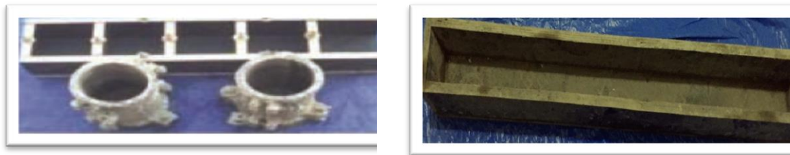
Figure. 2 Wooden molds for beam and cubes and plastic mold for cylinders
