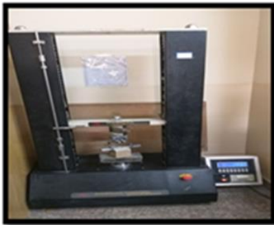
Figure 10. Three-point bending machine test.
