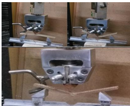
Figure 10. Three-point bending machine test.
