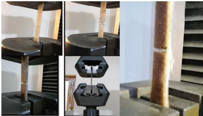
Figure 9. Tensile samples before and after failure during the test.
