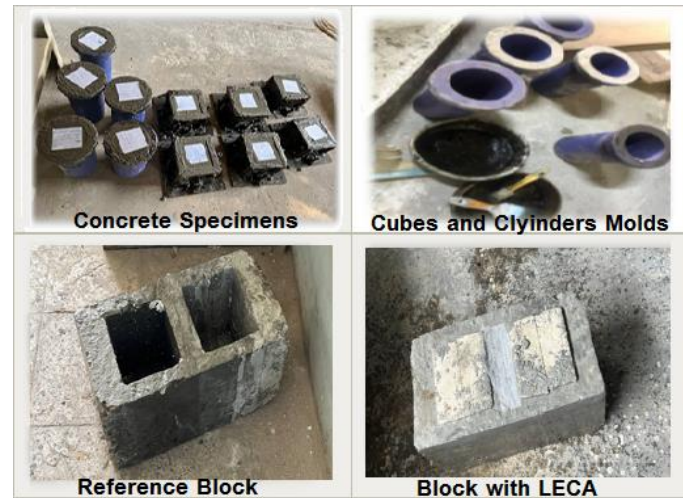
Figure 2. Molds and concrete hollow specimens.
