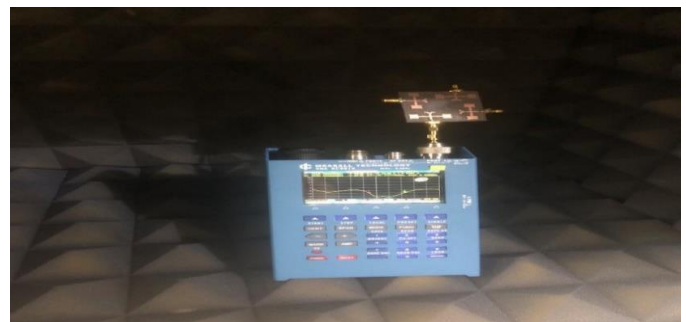
Figure 13. VNA Analyzer used to measure the S-parameters.
