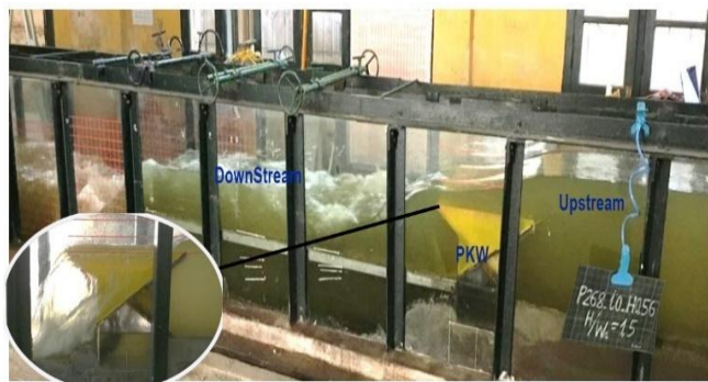
Figure 8. Experimenting on the Flow over PKW model at Vietnam Academy for Water Resources (VAWR)
