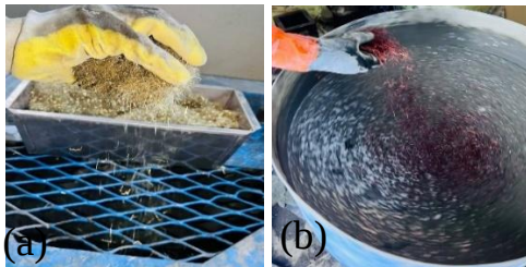
Figure 3. The method for incorporating (a) micro-steel fiber, (b) waste copper fibers.
