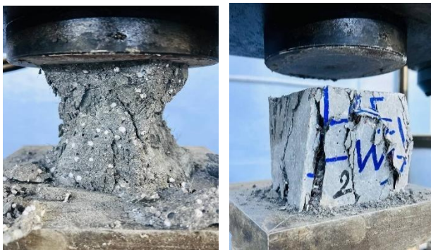
Figure 9. Compressive testing of the Cubes sample.
