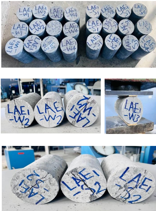
Figure 12. Samples subjected to the splitting test.
