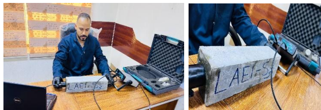
Figure 16. UPV test for A-EPSC samples.
