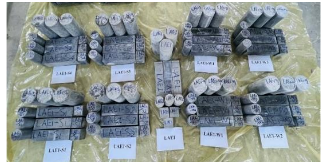
Figure 5. Prepared LWC samples for the tests.
