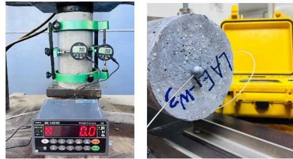
Figure 13. Modulus of elasticity tests (static and dynamic).
