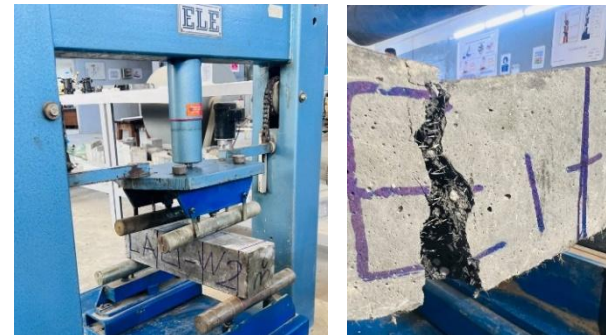
Figure 10. Bending strength and splitting strength of SLWC samples.
