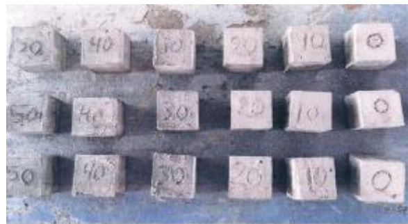
Figure 2. Specimens with cement replacement ratios and reference mix after demolding.
