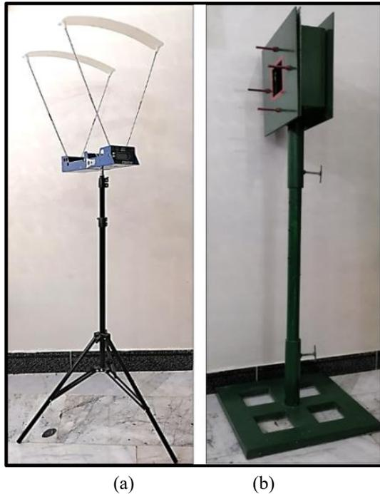
Figure 3. Ballistic test equipment:(a) Chronographs, (b) Specimen fixing tool
