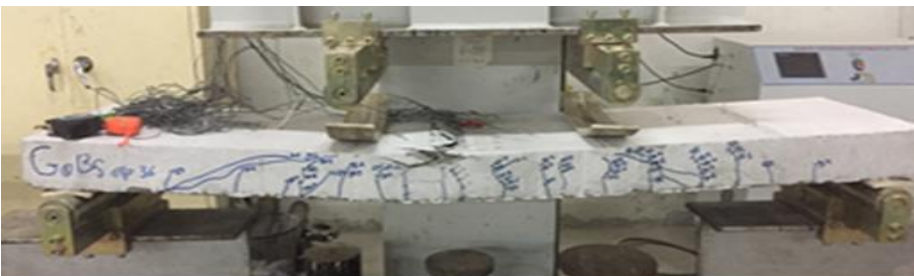
Fig. 10 Crack pattern and mode of failure of BS elp70
