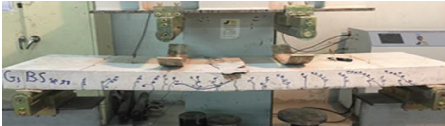
Fig. 8 Crack pattern and mode of failure of BS sp70
