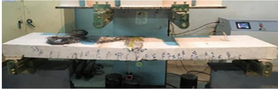
Fig. 7 Crack pattern and mode of failure of SS
