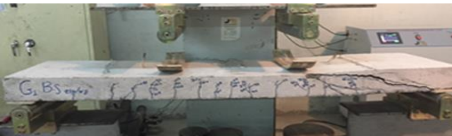
Fig. 7 Crack pattern and mode of failure of BS elp25
