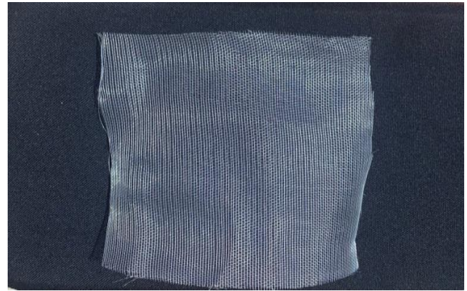
Figure 1. Aluminum alloy mesh.
